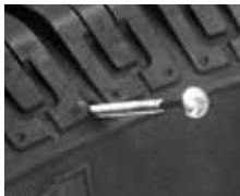
Puncture - Normally, the only evidence of a puncture will be a cut that extends from the tread of the tire through the inner liner.
