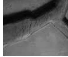
Cracking Between Tread
